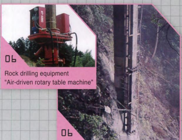
06 Bearing pile drilling (DHD method)
