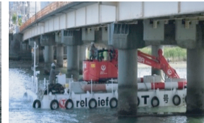
橋梁下空間で航行可能 Ability to pass under a bridge with overhead height
